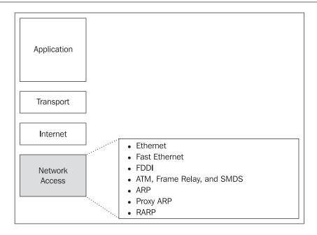
As you can notice, ARP and RARP are found at both the Internet and network access layers. Also, you can see that the TCP/IP network access layer contains LAN and WAN technologies that are found at the OSI physical and data link layers.
